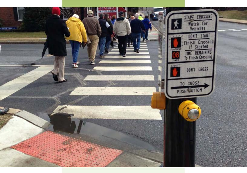
Pedestrian crosswalks, ADA ramps, pedestrian signals and push buttons are provided at the Market Street intersection. Note the water ponding at the ADA ramp. This is not unusual to find at even newly designed and constructed ramps.
