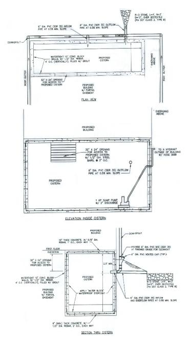
**Note:** Actual size and shape of cistern will vary depending on required amount of stormwater storage volume. This is an example. Actual design, size and shape may vary as long as function is met. External access must be provided with a lockable mechanism. All cisterns shall include structural design information for review prior to approval.
