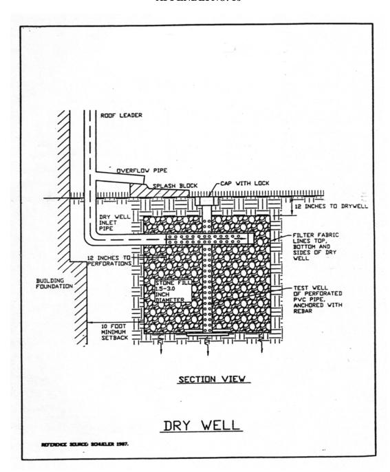
**Note:** An in-line sump with cleanout access shall be provided between the roof leader and the drywell/infiltration bed/leach ring or other similar infiltration facility. This is an example. Actual design, size and shape may vary as long as function is met.
